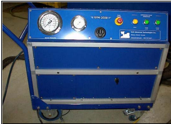
Fig. 7. A general view of the forced pulsed waterjet generator called the RFM (Retrofit Module). The enclosure contains all the controls to ensure safety at the workplace. The maximum power of ultrasonic generator in the RFM is 1.5-kW at 20-kHz.
