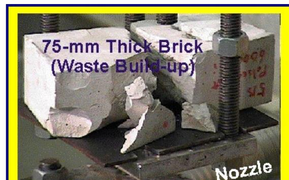
Fig. 17. A sample of brick (material to simulate chemical growth) fragmented by the pulsed waterjet generated at a discharge voltage of 10 kV (sample confined between steel plates).
