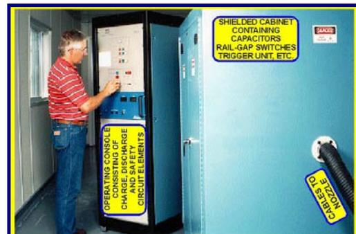
Fig. 3. A general view of the 2<sup>nd</sup> generation EPPS. Maximum stored electrical energy = 20 kJ at 40 kV.
