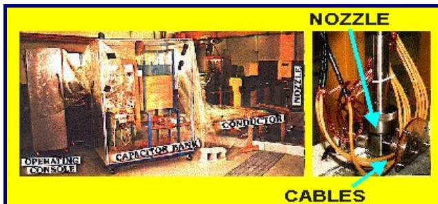
Fig. 2. The original (1<sup>st</sup> generation) electrical pulsed power system (EPPS) fabricated from scratch to investigate the feasibility of generating pulsed waterjet. Maximum stored electrical energy = 5 kJ at 40 kV.
