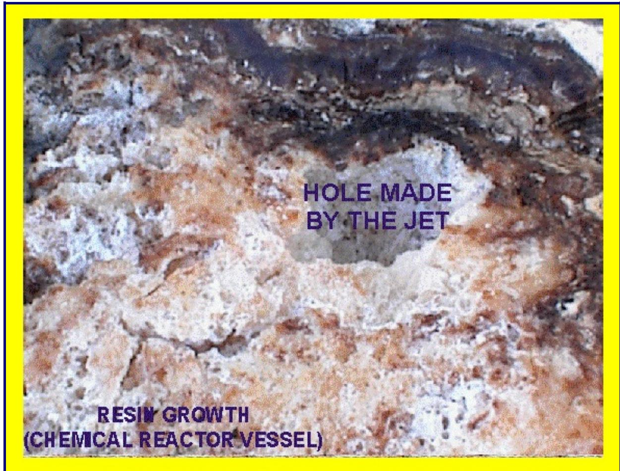
**Fig. 18. Hole and fractures made in the chemical resin (unwanted growth) with the pulsed waterjet generated by the discharge. Water pressure = tap water (0.5 MPa), Nozzle diameter = 9.52 mm, Voltage = 6 kV and  $E_0 = 7.4$  kJ.**
