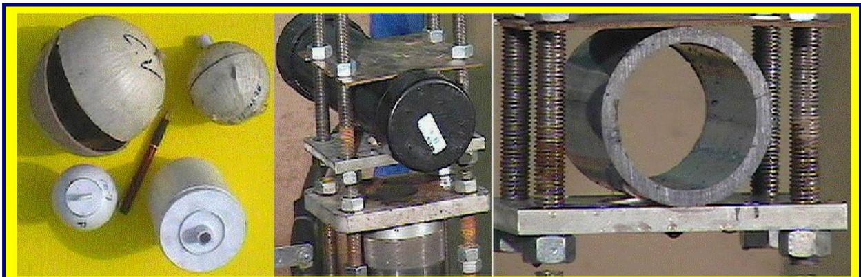
**Fig. 11. Pipe bombs of various shapes and sizes. The materials of the pipes vary from brittle to plastic. The types shown on the left are known as pyro ammunition the containers fabricated from plastic, paper, etc.**
