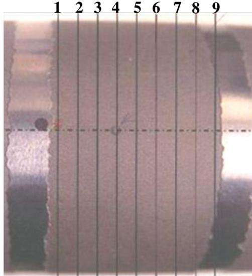
Fig. 8. Measurement of residual stresses at the stripped sections shown by X-ray Diffraction (XRD) technique (see the Table below).
