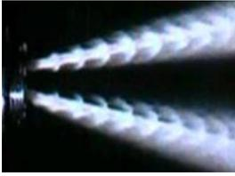
Fig. 1. General appearance FPJ at 20-kHz issuing from a Twin-orifice rotating nozzle.
