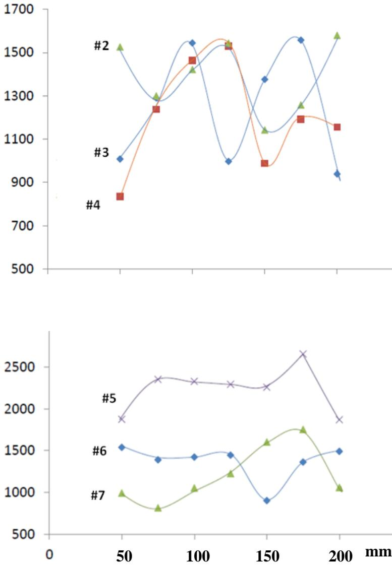
Fig.5. Variation of microhardness (Vickers) along the length of the pins.
