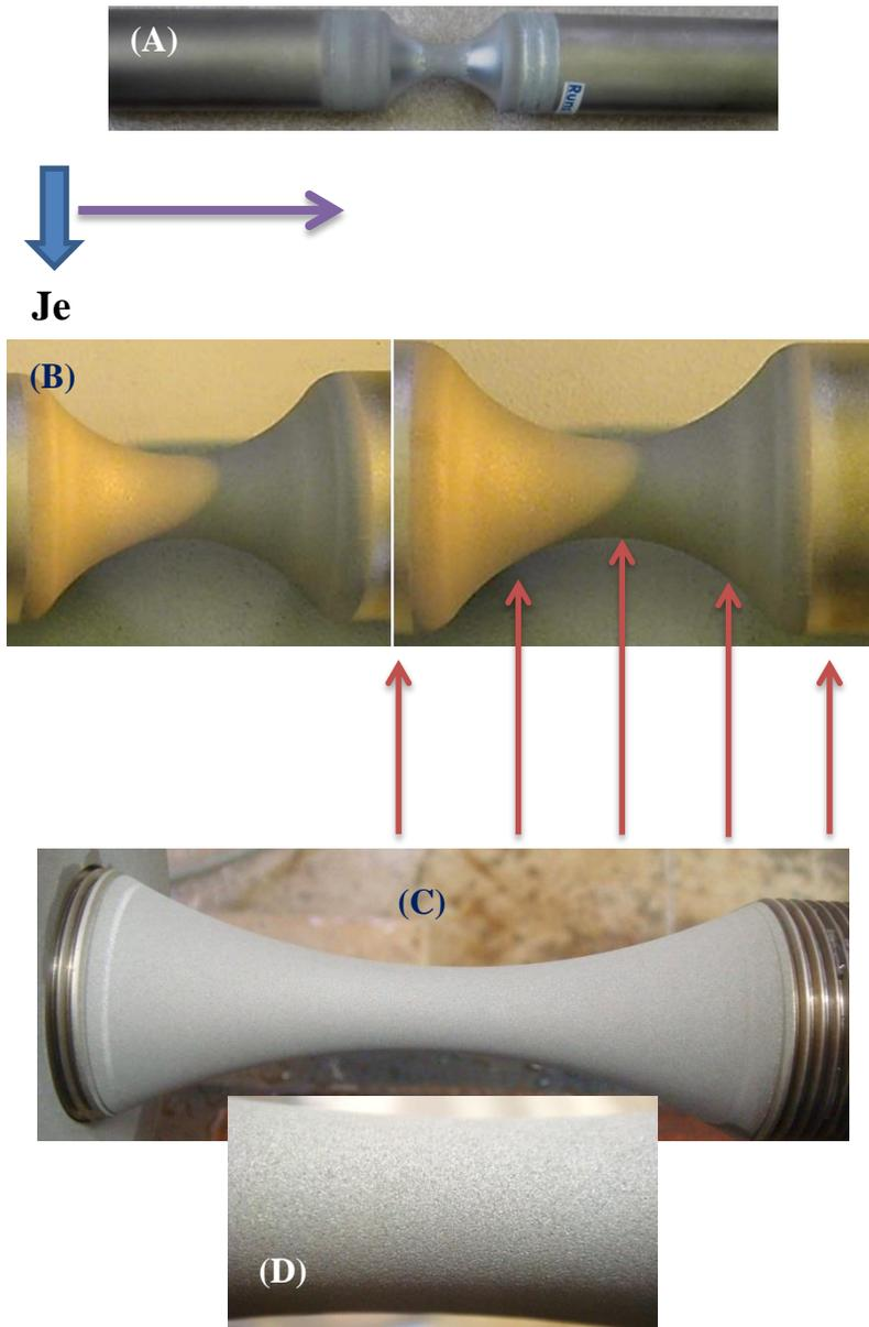
Fig. 9. Fatigue tests conducted on stripped fatigue bars. (A) Unconventional fatigue bars, (B) Tests conducted on ad-hoc basis ( $S_d$  not varied as the jet traversed from one end to the gage section). Results are summarized in Table 1, (C) Tests conducted on hour-glass fatigue bars (19, 26) fabricated according to ASTM standard (31). Sample results are summarized in Table 1.
