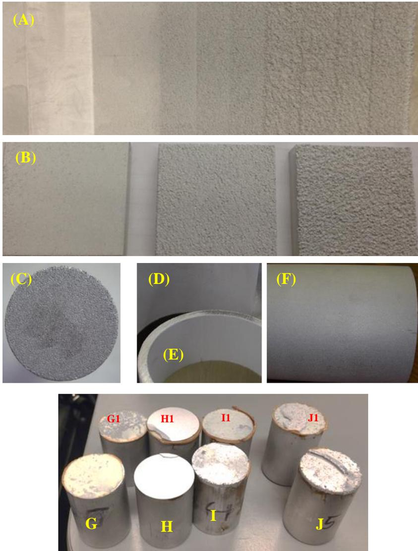
Fig. 10. Prepping substrate materials with the CWJ and FPWJ for measuring bond strength of the coatings (work in progress; see Ref. 63).
