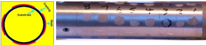
Fig. 3. Stripping the HVOF coating from the periphery of the cylindrical pins for SCM study.
