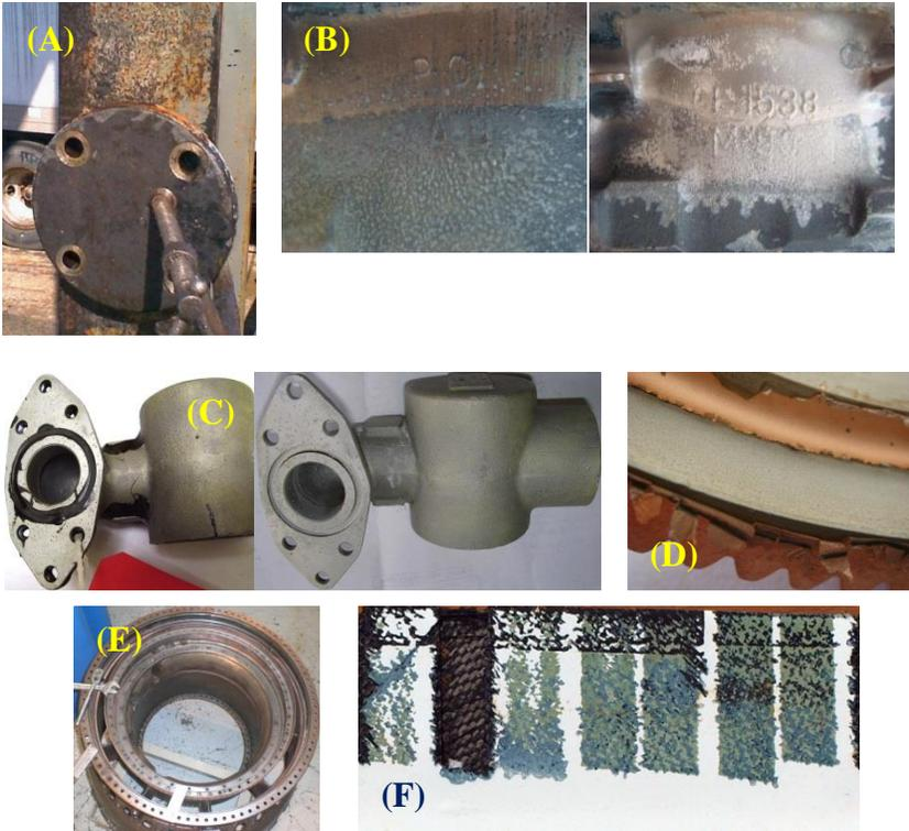
Fig. 2. Photographs showing the efficacy of the FPFJ in processing the surfaces. (A) Rust from infrastructures, (B) Corrosion from turbine blades, (C) Epoxy and (B) Elastomer coatings and seals from helicopter components, (D) Copper from helicopter parts, (E) Thermal barrier coatings from aircraft engines and (F) epoxy coatings from composite surfaces.
