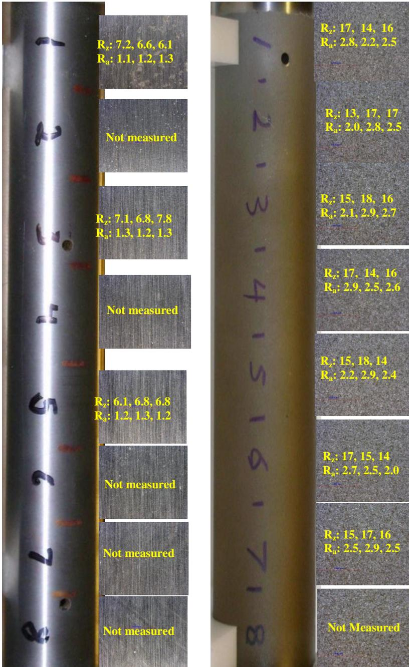
Fig. 6. General view of the cylindrical pin #5 (Fig.5) before and after stripping to show the effect of microhardness of the coating.  $\tau \approx 0.076$
