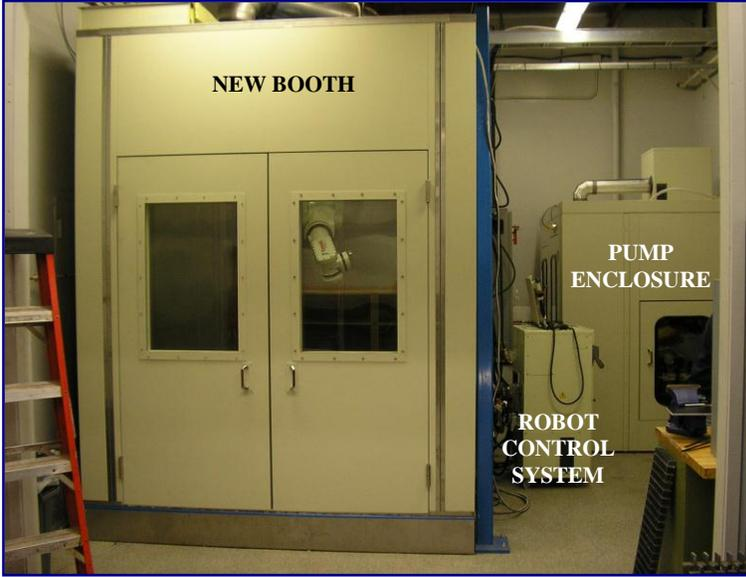
Fig. 8. A general view of the new booth with well insulated walls.
