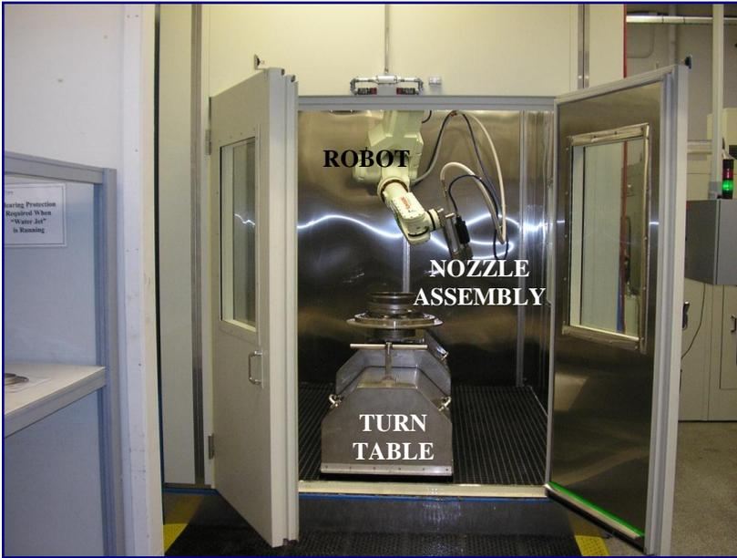
Fig. 10. Interior view of the booth manufactured with stainless steel, acoustic materials and double-pane windows to abate noise levels when the system is in operation.
