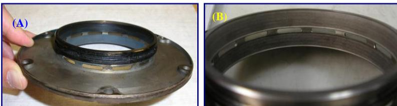
Fig. 14. Plasma sprayed part. (A) Prior to stripping and (B) stripped with the APWSS.
