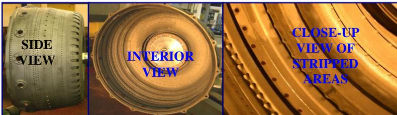
Fig. 13. One of the several engine parts stripped in the APWSS at pressures  $\approx 69$ -MPa.
