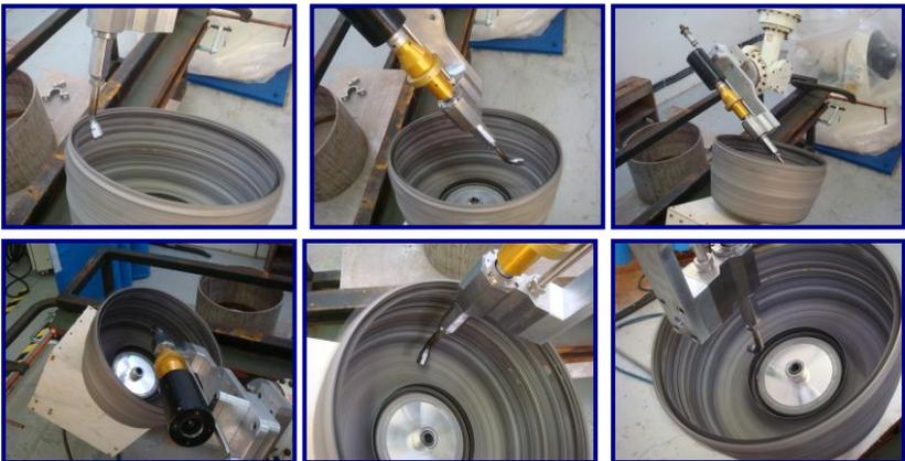
Fig. 5. Programming the robot (based on simulation studies) to strip critical areas (from top to the bottom) of one of the engine components without damage.
