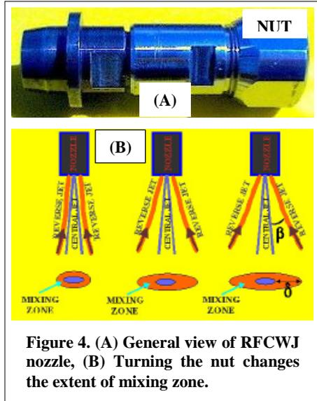
**Figure 4. (A) General view of RFCWJ nozzle, (B) Turning the nut changes the extent of mixing zone.**
