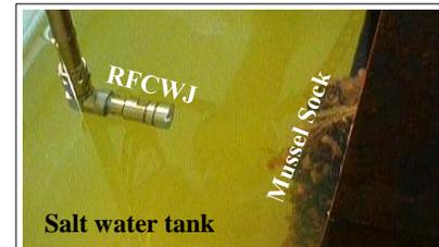
**Figure 7. Salt water tank showing the RFCWJ nozzle positioned over the infested mussel sock.**
