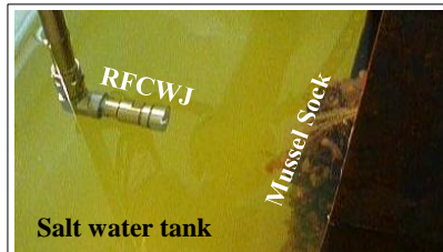
Figure 7. Salt water tank showing the RFCWJ nozzle positioned over the infested mussel sock.
