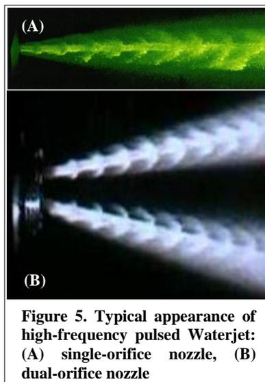
**Figure 5. Typical appearance of high-frequency pulsed Waterjet: (A) single-orifice nozzle, (B) dual-orifice nozzle**
