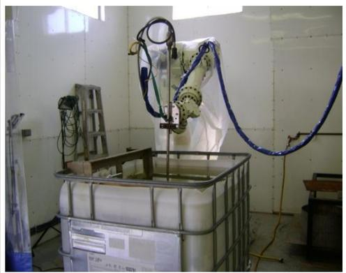
**Figure A1. A general view of the experimental set-up using the robot for manipulation of the nozzle.**
