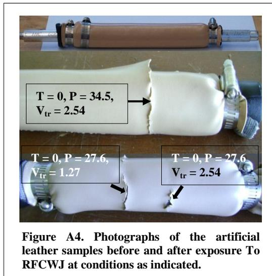
**Figure A4. Photographs of the artificial leather samples before and after exposure to RFCWJ at conditions as indicated.**
