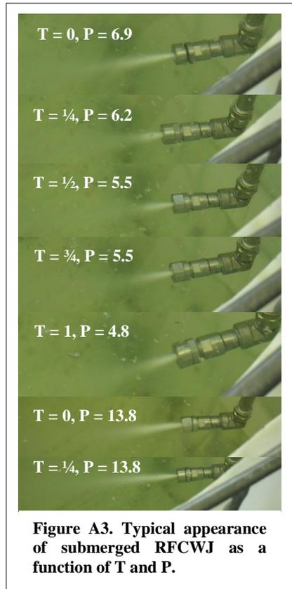
**Figure A3. Typical appearance of submerged RFCWJ as a function of T and P.**
