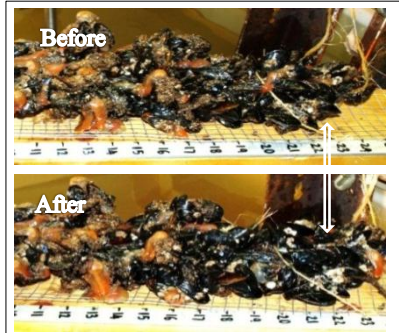
Figure 8. Appearance of the sock after testing at 6.9-MPa.
