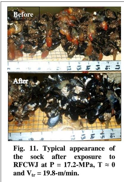
**Fig. 11. Typical appearance of the sock after exposure to RFCWJ at  $P = 17.2$ -MPa,  $T \approx 0$  and  $V_{tr} = 19.8$ -m/min.**
