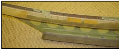
Fig. 4. Removing HVOF coating (specification not known) from aircraft frame.
