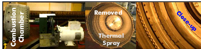
Fig. 7. Removing thermal spray barrier coating from the inside surface of a combustion chamber.
