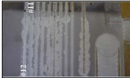
Fig. 1. Removal of 1.27-mm thick HVOF (WC-Co) coating from steel substrate at 103.5-MPa at various traverse speeds (tests conducted for a US airline).
