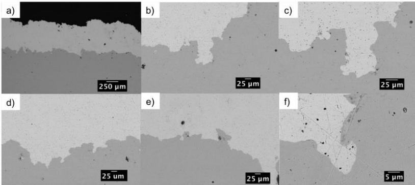
**Fig.3. Cross-sections of coating/substrate interfaces at different magnifications; (A) (B) (C) are FPWJ-2 and (D) (E) (F) are FPWJ-5 samples.**
