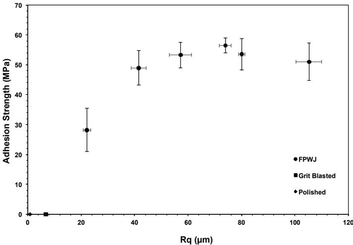
**Fig. 4. Coating adhesion strength vs. substrate quadratic mean roughness.**
