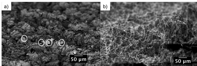
**Fig.5. Fracture surface topography of the FPWJ-2 sample; (A) substrate side and (B) coating side. Copper residues that remained on steel surface are circled.**
