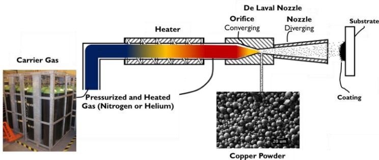
**Fig.1. Cold Spray process.**
