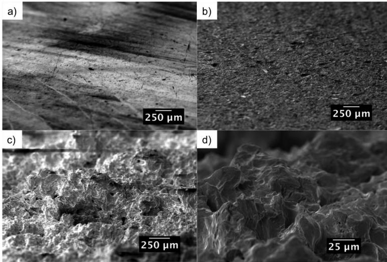
**Fig. 2. Substrate surface topography obtained using different surface preparation methods; (A) polished, (B) grit blasted, (C) FPWJ-2, and (D) FPWJ-2 details.**
