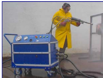
Fig. 11. Model 69-MPa RFM (retrofit module) 20-kHz pulsed waterjet generator.
