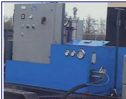
Fig. 10. The current FPWJ machine designed and manufactured for use with multiple-orifice nozzle assemblies.
