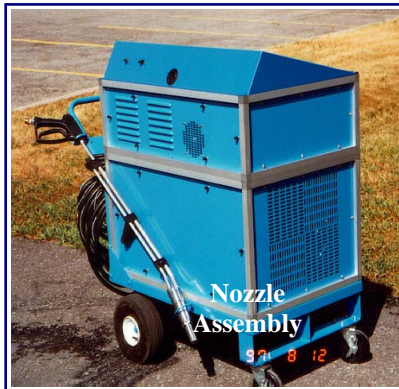
Fig. 8. The first FPWJ machine manufactured in 1996-97, using magnetostrictive transducer located inside the nozzle assembly (single-orifice).
