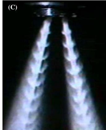
Fig. 1. (A) Method of generating FPWJ by placing a microtip (probe) inside a regular nozzle (1). (B) Structure of FPWJ emerging from a single-orifice nozzle assembly and (C) Structure of FPWJ emerging from a dual-orifice rotating or non-rotating nozzle assembly.
